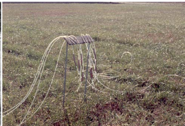
Vacuum probes with thin plastic tubes connected through the top stopper. The leaching of nutrients is monitored for each plot every week over a three-year period.
