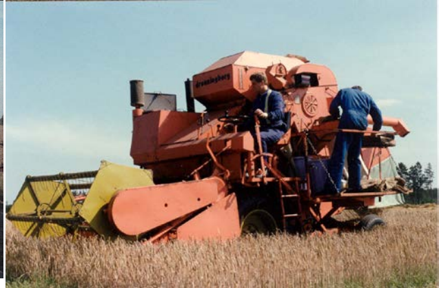
A mini harvester in use. The crop on individual plots are collected and measured.
