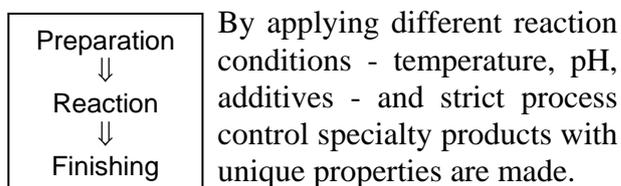
These specialty products are named modified starches. They still retain their original granule form and thereby resemble the native (unmodified) starch in appearance, but the modification has introduced improved qualities in the starch when cooked. The paste may have obtained improved clarity, viscosity, film-forming ability etc.
